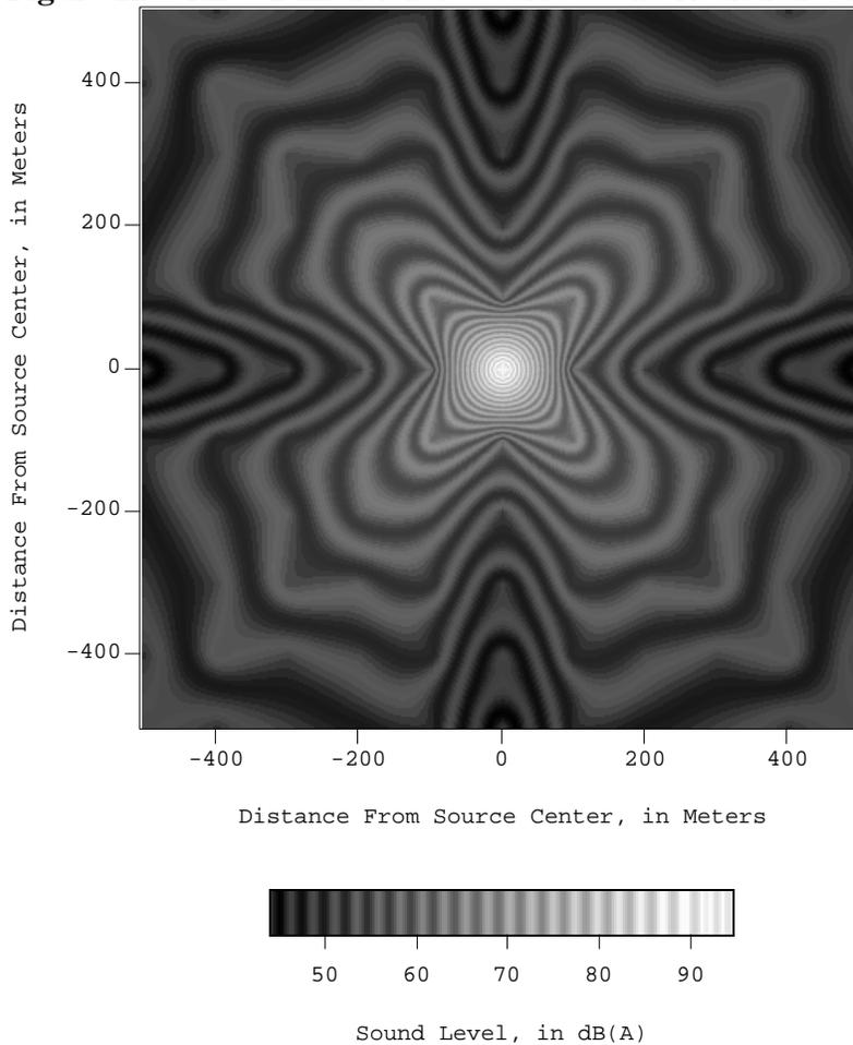
The substantial departure from the results observed in the omni-direction point model are clear. The strong bands of sound radiated toward the corners of the cube (45, 135, 215 and 305 degrees) are related to largest observable surface area at the sound receptor (two wall surfaces are visible by the sound receptor) while less of the source area is observable in other directions.
