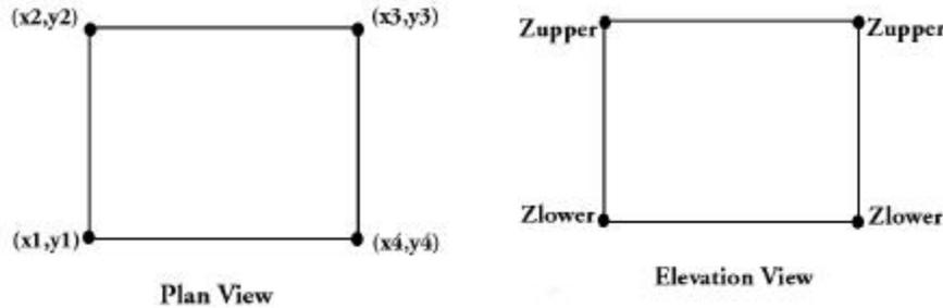
The 3-D distribution of points for surface sources is determined as follows:
