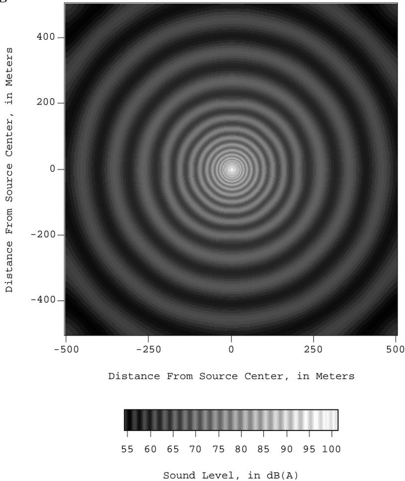
Presented in Figure 11 is the plan view of a sound source represented by 3x3 arrays of points located on the surface of the “cube” with barriers behind them. The results of the directivity analysis of the 3-D representation are shown in Figure 12.
