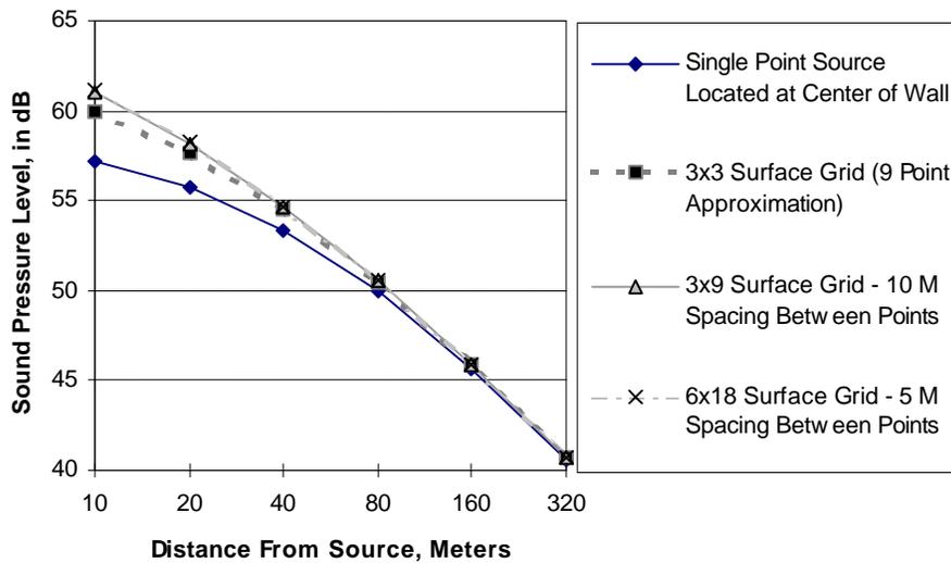
The ISO 9613-2 engineering method requires that all sound sources must be defined as point sources. For large sound sources that are closer to the receiver than twice the diameter of the relevant area of sources, or when the source is partially blocked by a barrier, the standard says the source must be broken down into several points.
