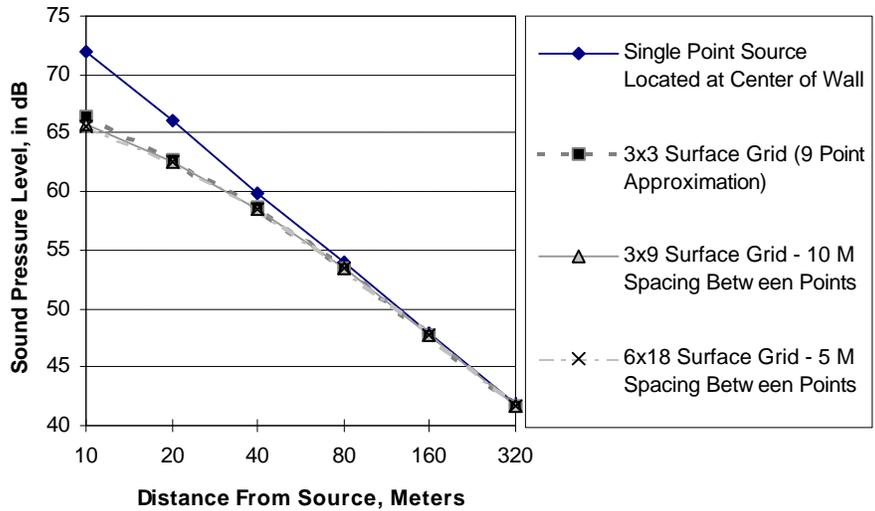
**Figure 6.**  $L_p$  As A Function Of Parallel Distance From A 90 M X 30 M Wall
