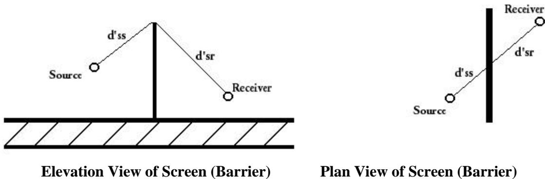
The screening attenuation ( $D_z$ ) is calculated with the following equations:
